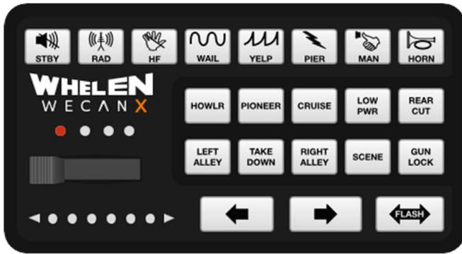
**Slide 1:** Activates rear facing lighting with a synced triple flash “comet flash 75” pattern. All red alternate with all blue. The Tail Light Flasher is activated flashing the brake and reverse lights.
